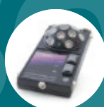
Tightness and sealing control: Ultrasonic emitter with 13 emitters LKSDOME
