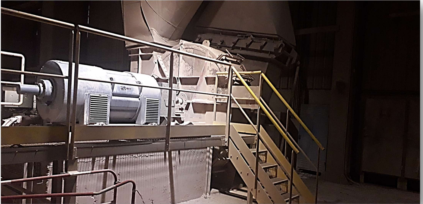
Cement plant industrial smoke exhaust blower/fan (1480 RPM- 650 kW)
